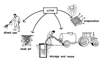
Figure 2: Options for re-use of urine from ecosan. [Illustrator: Hans Mårtensson; Source: Esrey et al, 1998]
